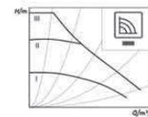
Recommended for systems with fixed system resistance requiring a constant volume flow and for replacement of AC pumps.
